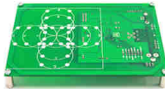
Pi941 Multiprotocol Reader Proprietary reader module for SIC9410, SIC9311 and SIC9100 ICs
