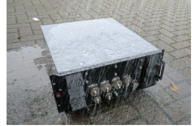
P4898R water ingress test
